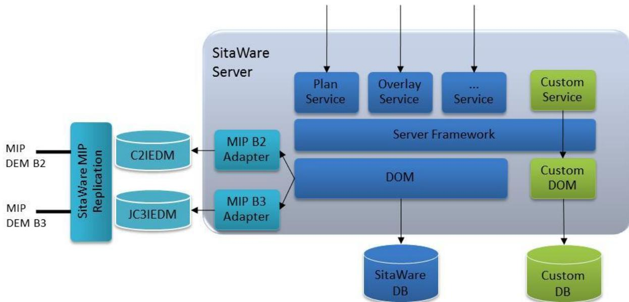
**Figure 2, An example of an architecture with an external MIP interface and different ways to extend to eg. simulation systems**
