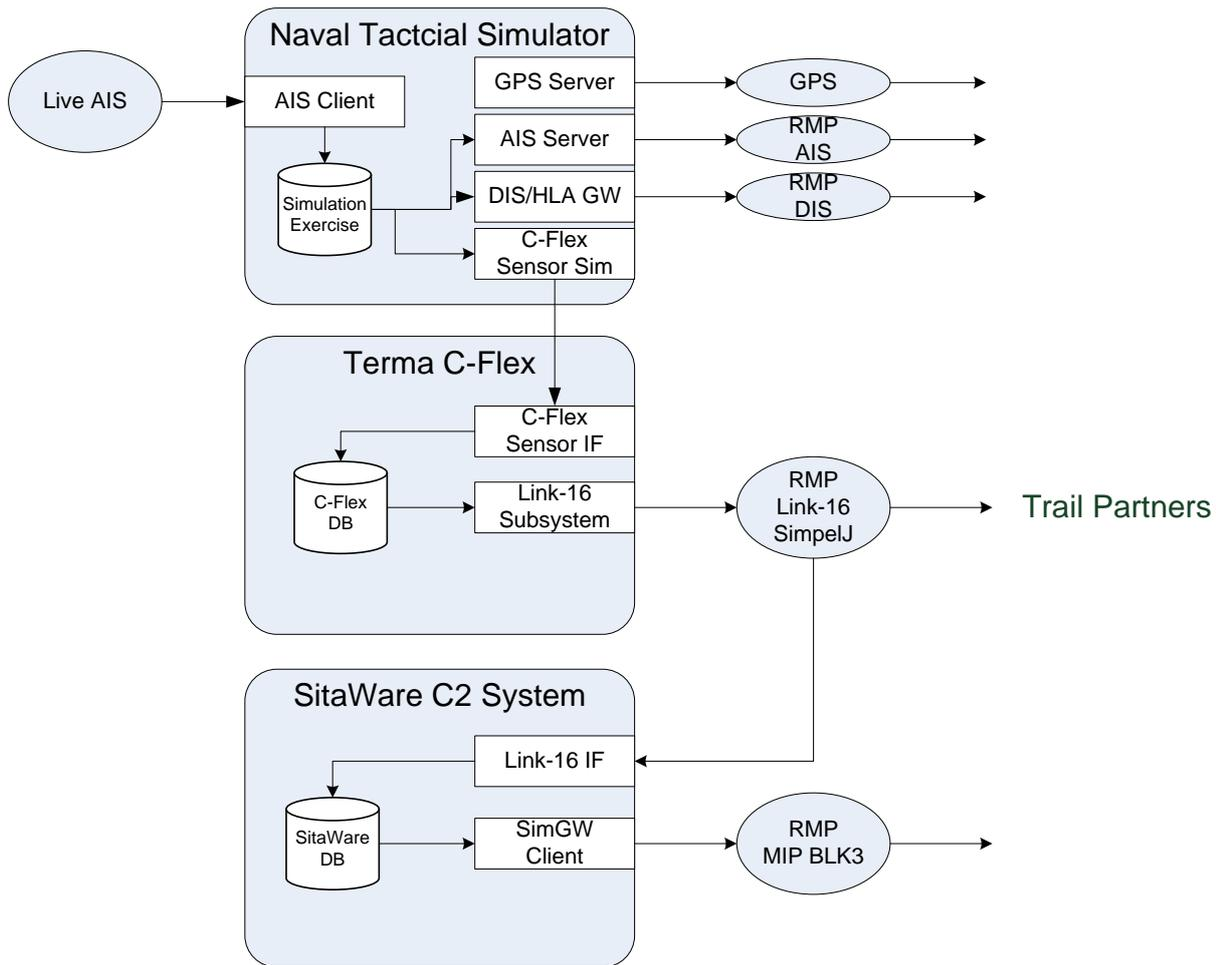
**Figure 6, Simulation to C2 example from CWIX 2012 enabling the simulated maritime picture to be shared among joint coalition partners using MIP**
