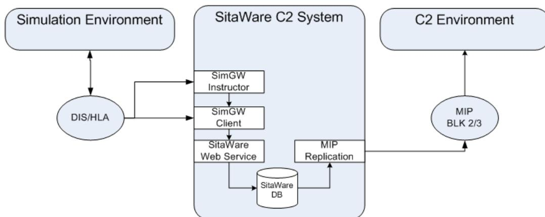
**Figure 4, An example SitwWare SimGW based simulation to C2 gateway via MIP.**
