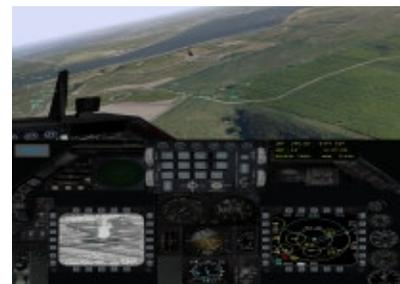
**The FAC/JTAC Trainer (IFACTS)** - is a deployable, PC-based system for training and practising the direction of close air support, providing a synthetic environment within which the FAC can control aircraft missions using simulated communications and simulated equipment. Equipment includes GPS, ground laser target designators, laser range finders, binoculars, NVG, compass, thermal equipment and ROVER.
